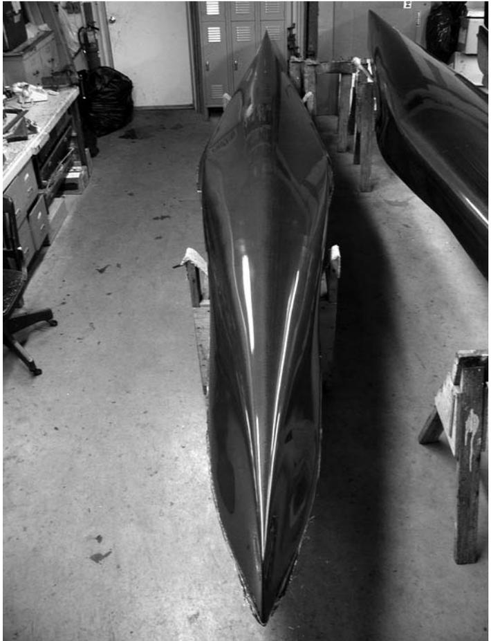
Above: The bottom side of a *V-1M* (looking from the stern) and below, the bottom side of a *Hassel* looking from the stern — at **Crozier’s** shop. Of all the pro boats reviewed, the *Gillies* is easiest to distinguish upside down(!) with its hard chine (see small picture from **Matt Streib** to the left).
